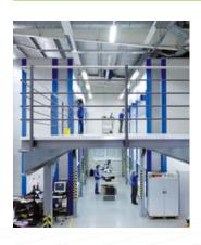
Vertical Lift Modules can be built through several floors with up to 6 access openings placed on the front or rear side of the unit. A mezzanine floor can be installed to enable operation on several levels at the same time (with loading at one level or side and retrieval at the other).
