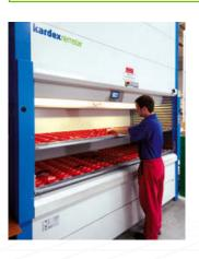
A dual tray delivery option makes it possible to use two work levels in the access opening. A tray is delivered into the first work level in the access opening and the shutter door closes. While items are stored or removed, the next tray is being retrieved and kept in a waiting position behind the access opening, decreasing wait time even further.
