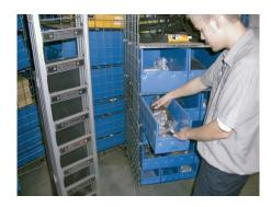
**Put/Batch Lights:** Used with both horizontal and vertical carousels, as well as VLMs, these light-directed picking modules direct an operator to put or store items in a specific or active location when replenishing stock. They can also be used for order consolidation, batch picking and sortation at workstations located near the automated storage and retrieval units.
