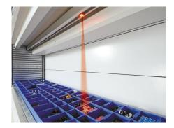
**Position Indicator Light Bar:** Incorporated into the access openings of both vertical lift modules and vertical carousels, these LED lights illuminate in alignment with the position of the required item where it is stored in the tray.
