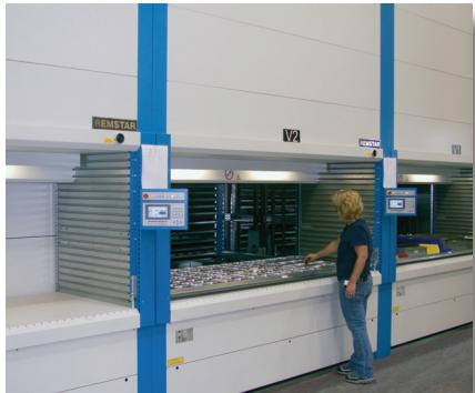
*The three Shuttle VLMs were installed in the workzones where the modules are built. With the shelving condensed into the VLMs the free floor space was used for a value generating module assembly area while the parts were kept close at hand.*
